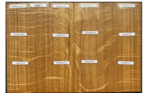
Figure 4: Evaluation chemical resistance on oak
