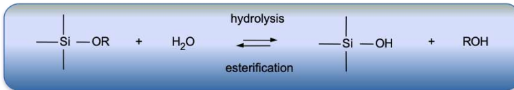
Figure 12: Hydrolysis of the ethoxysilane groups
